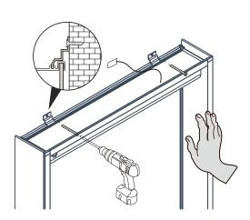
Top mounting brackets must be attached to furring strip/channel or wall studs.
