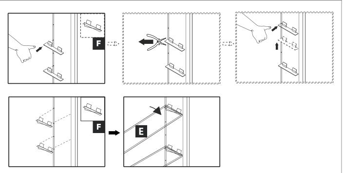
1.Insert clear snap in shelf clips (F) into holes on the sides of the cabinet.
