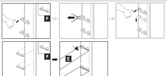
1.Insert clear snap in shelf clips (F) into holes on the sides of the cabinet.
