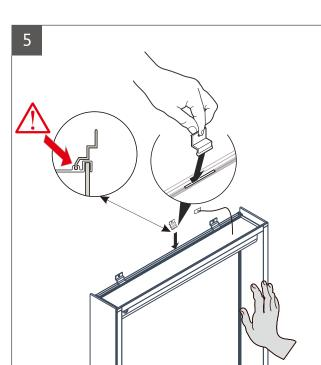
Insert top mounting bracket into the top of the cabinet.
