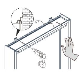
Top mounting brackets must be attached to furring strip/channel or wall studs.
