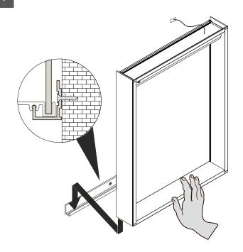
With assistance, to rest the cabinet on the mounting bracket and hold in place.
