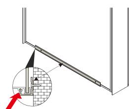
Make sure cabinet is leveled and fully inserted into the groove of the bottom bracket.
