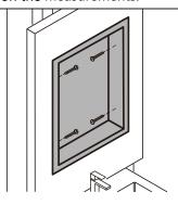
Affix using hardware screws into the studs.
