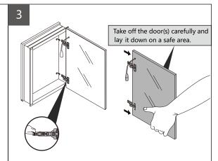
While supporting the door release (the lever under the hinge arm), slide the door off the frame.
