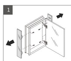
For recess mount only! Carefully remove side mirror panels for recess mount installation.
