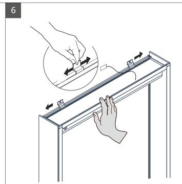
Make sure top brackets are locked in the grooves.
