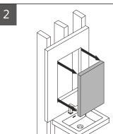
Cut the marked perimeter with suitable tool.
